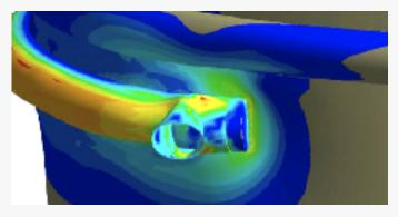
**NOZZLE LOADS:** Detailed evaluations to understand and mitigate stresses within pressure vessel nozzles.
