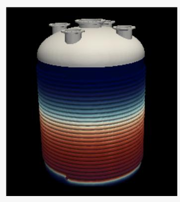
We combine finite element analysis with CFD to analyze both the fluid dynamics and structural integrity of reactors under operational conditions. While CFD models fluid behavior such as heat and mass transfer, FEA assesses thermal stresses and deformations on the reactor's structure. This integrated approach ensures optimized reactor performance and durability under real-world conditions.
